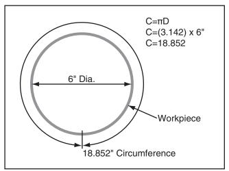
Figure 22. Calculating circumference example.
